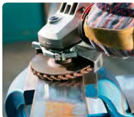
Professional derusting and descaling
