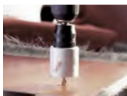
HSS bi-metal with 8% cobalt. Progressive tooth strip.
