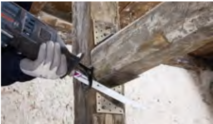
The progressive tooth pitch is ideal for sawing thick wooden beams containing thin fixing elements.
